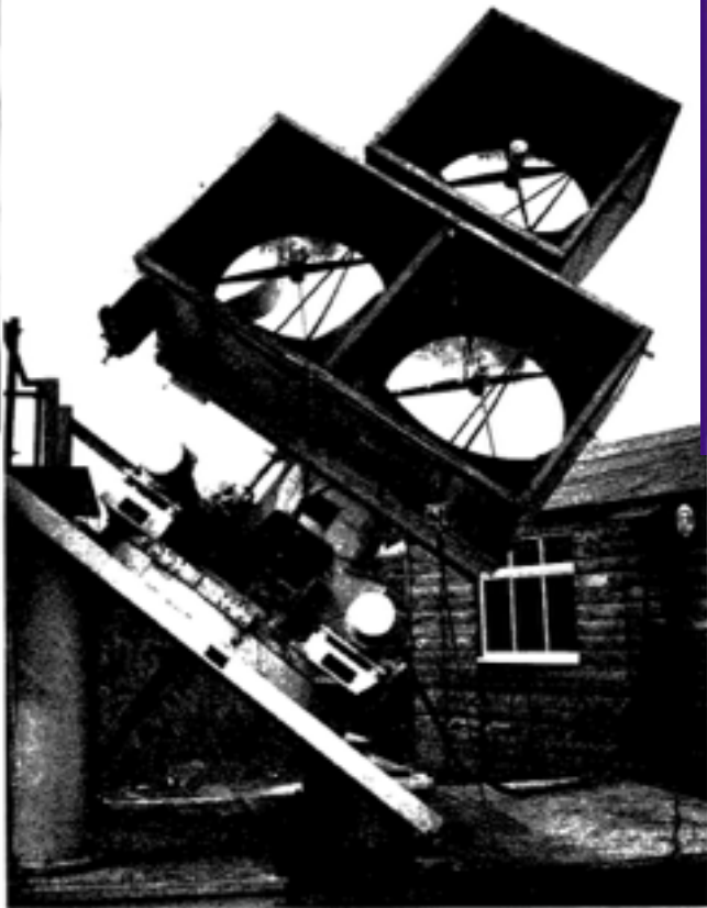
The existing light receiver installation at A.E.R.E., Harwell. The bank of three-foot f/10 mirrors is mounted equatorially for drift scans.
